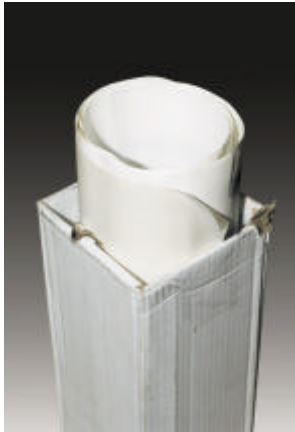
Graphics masked with ordinary application tape are prone to wrinkling, tunneling and edge curling, especially when rolled!
