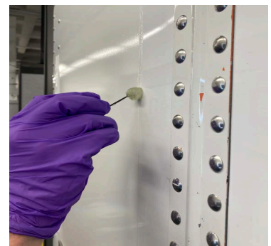
Figure 6. Applying Edge Sealer
