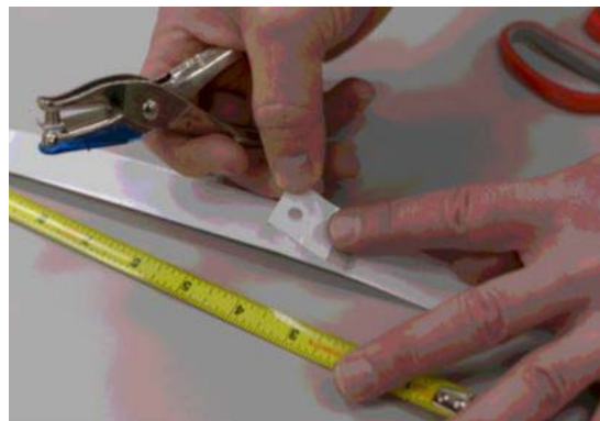
Figure 1. Preparing the test strips
