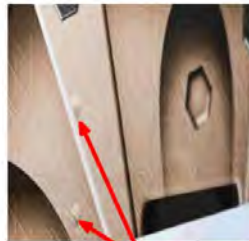
Tenting over rivets even on relatively flat surfaces.
